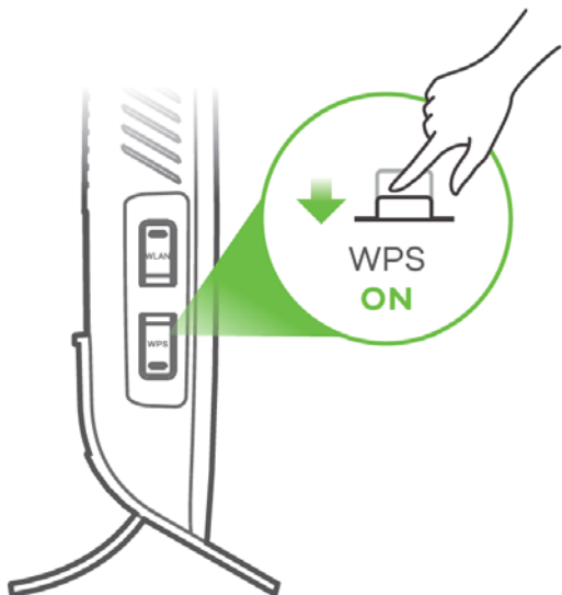
Figure 36 WLAN / WPS Buttons on the Right-Hand Side (EMG3525-T50C)
