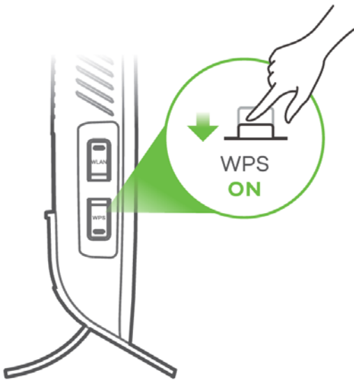
Figure 31 WLAN / WPS Buttons on the Right-Hand Side (VMG3625-T50C)
